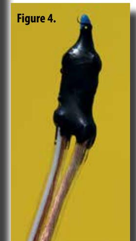
11. Put some hot water in the other container, and put the thermistor into the water. Wait about ten seconds, then measure the voltage as in Step 9. Check the temperature of the water with the thermometer, and record the voltage and temperature in the Calibration Table.
