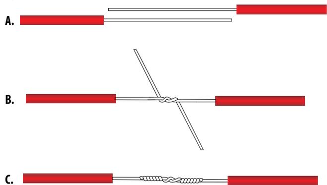
The Western Union Splice. Bring ends of wires to be spliced together so that the ends are pointing in opposite directions (A). Twist each wire 3/4 of a turn in opposite directions (B). Turn the ends so they are at right angles to the wires being spliced, and twist each end to form at least five more turns spaced as tightly as possible (C). It is easier to make these twists with a pair of needle-nose pliers. Cut off the ends and twist them close to the center wire.
